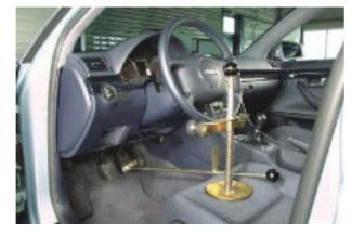
The support plate is then pulled up along the shaft until comes into contact with the front of the seat. Apply the brake pedal by pushing down on the shaft using the round knob on the end of the shaft to assert pressure on the brake pedal.
