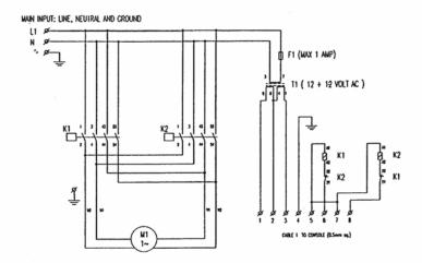
The motor is 1.5kW and needs to be fused by 16 Amp. slow acting.
