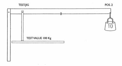
With 20 Kg mounted in Pos.2 the display will indicate 200 Kg (+/- 6 Kg).
