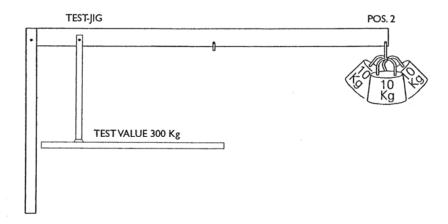
If the brake tester indicate values outside of this tolerance, you must adjust the gain trimmer on the I/O board in the cabinet. After many gain adjustments you must check the zero adjustment.
