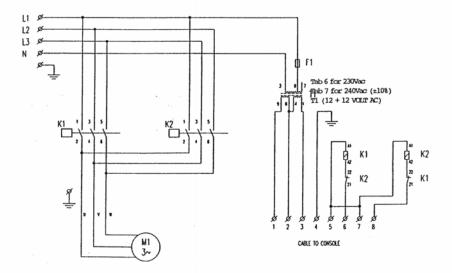
The motor is 1.5kW and needs to be fused by 10 Amp. slow acting.
