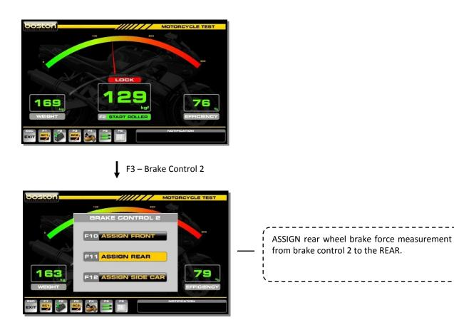
After the brake force measurement has been assigned for the rear wheel, the operator should again test the rear wheel for brake force fluctuations. Follow the same Brake Force Fluctuations procedure as was done for the front wheel.
