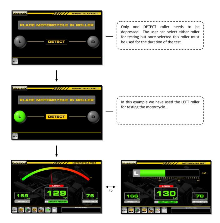
The motorcycle layout displays are a little different from the standard layouts. This is because there are no LEFT and RIGHT readings as motorcycles only have FRONT and REAR readings (and sidecar if fitted). This display shows a single scale to display the force from a single brake system, the weight obtained from the wheel being tested and the efficiency result at the end of the test.
