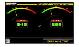
If wheel lock is achieved, the LEFT and RIGHT indicators will show. If wheel lock cannot be achieved, the software will automatically stop the rollers when stable readings have been measured for 3 seconds.
