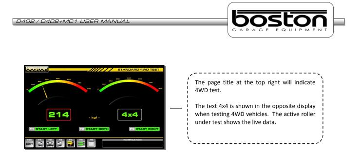
During the testing of the FRONT LEFT wheel, the text 4x4 is shown in the right side results box. The right side roller is also operating but in the reverse direction.
