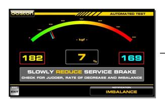
The software now checks for IMBALANCE. The user must SLOWLY APPLY THE SERVICE BRAKE until the force from either wheel reaches 75% of the maximum force achieved in the previous SERVICE BRAKE test. The red needle indicates this value and when reached, an audible bleep is sounded by the software. If wheel lock is achieved during this test the software automatically restarts the rollers.
