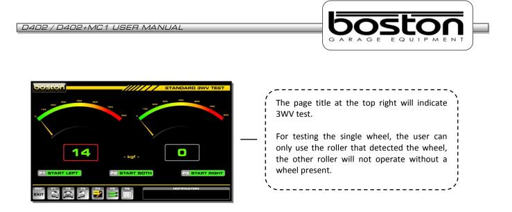
After testing the single wheel, the user should save the test result to the relevant axle in the same way as for the standard test.
