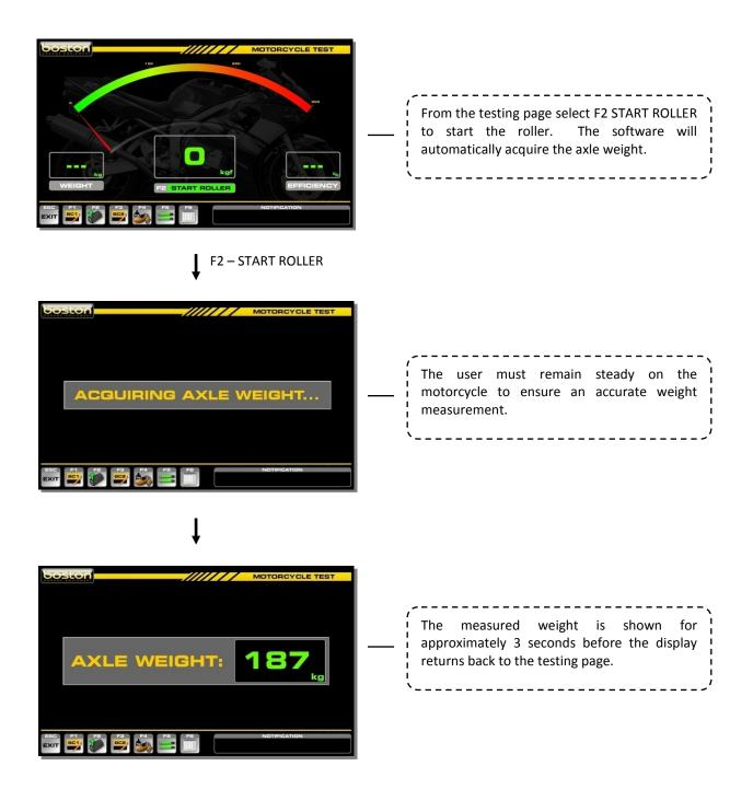
As before, the user is alerted to the rollers starting by means of the audible buzzer and the flashing red indicators on the display. When the roller starts, carefully position the wheel in the centre of the roller before applying the brake. This is important with larger / heavier motorcycles as they can be difficult to handle.
