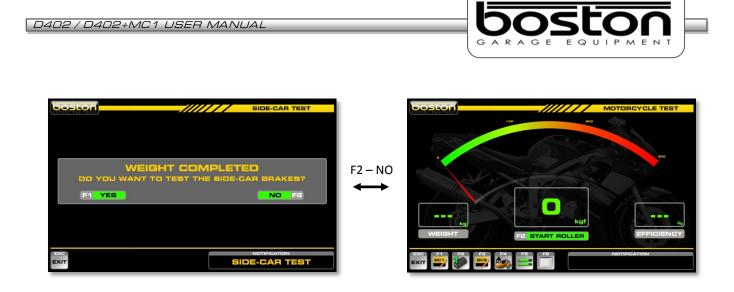
After the sidecar weight has been acquired, the operator can choose to test the sidecar brake (if fitted and controlled by either BC1 or BC2).
