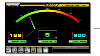
The rollers have started and brake effort is gradually applied. Both readings for LEFT and RIGHT can be seen together in both digital and analogue format using two different colour needle pointers. This gives a good indication of severe imbalance if present.
