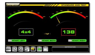
During the testing of the FRONT RIGHT wheel, the text 4x4 is shown in the left side results box. The left side roller is also operating but in the reverse direction. In this display layout, the analogue needle pointer is removed from the inactive measurement display.
