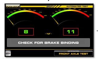
The operator should now check for binding from either wheel.
