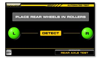
As before, the software detects the wheels and automatically weighs the axle.
