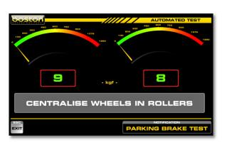
Once the SERVICE BRAKE test is complete the PARKING BRAKE must be tested. With the rear axle still positioned in the roller bed the rollers will re-start.
