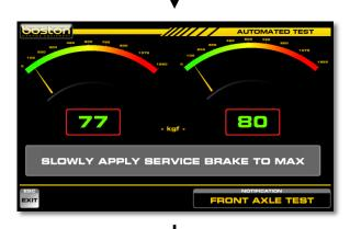
An audible 'bleep' will sound and the operator must now apply the SERVICE BRAKE to max.
