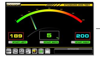
The rollers have started. Both readings for LEFT and RIGHT can be seen together in both digital and analogue format.
