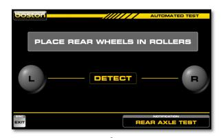
Drive the vehicle forward and place the rear axle into the roller bed.
