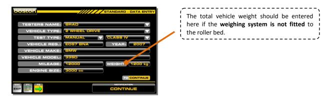
The software will acquire the axle weight automatically when the user starts either roller for the first time for each axle. The message ACQUIRING AXLE WEIGHT is shown while the system checks for a stable weight. The acquired axle weight is shown shortly after. See screenshots below are in sequence. Once the weight has been acquired the software reverts back to the testing page and the selected roller(s) will start. There is an audible warning and warning text in red to alert the user.
