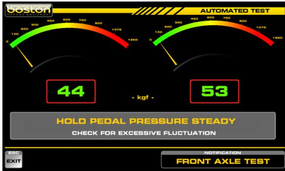
The pedal pressure must be held steady until instructed to release.
