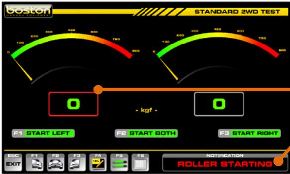
In this example, the left roller has been selected. There is an audible buzzer and three flashes of the red box to alert the user. The message 'ROLLER STARTING' is also shown in the notification box.
