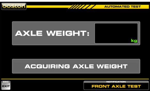
The software waits for a few seconds to allow the vehicle to stabilise in the rollers before the weight measurement is taken.
