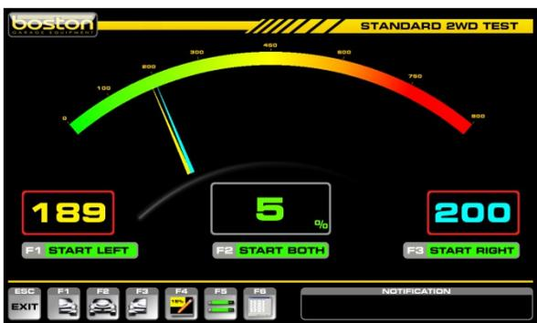
The rollers have started. Both readings for LEFT and RIGHT can be seen together in both digital and analogue format.
