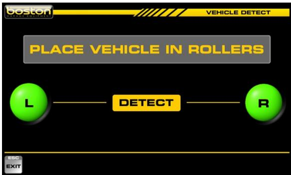
Both wheels have been placed in the rollers as shown by the two green indicators. This page is shown only for a few seconds before the software moves on to the vehicle testing page.
