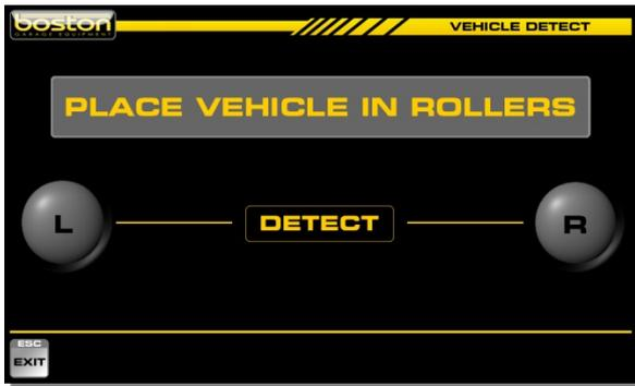
At this point the software is waiting for the first axle to be placed in the rollers. The two grey circles indicated as 'L' and 'R' will turn green when the respective detection roller has been depressed by the wheel.
