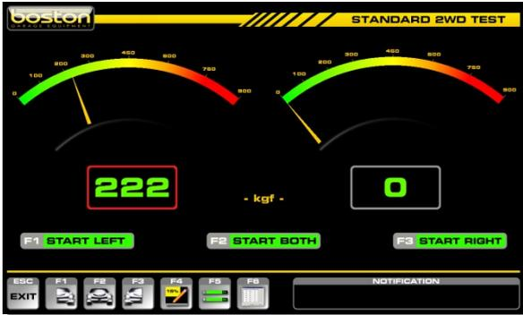
Left roller is running and brake force is being slowly applied.
