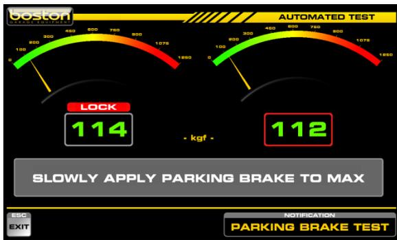
An audible 'bleep' will sound and the operator must now apply the PARKING BRAKE to max.
