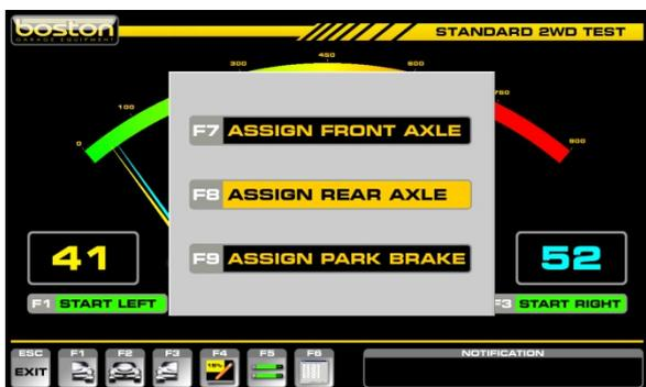
Select F8 to assign all the results from the REAR AXLE test to memory.
