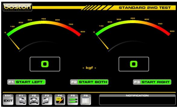
From the testing page select F1, F2 or F3 to start the rollers. The software will automatically acquire the axle weight.
