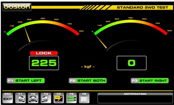
Left roller has stopped due to wheel lock. The wheel-lock indicator is shown above the corresponding reading. The highest brake force reading achieved is shown in the results box.
