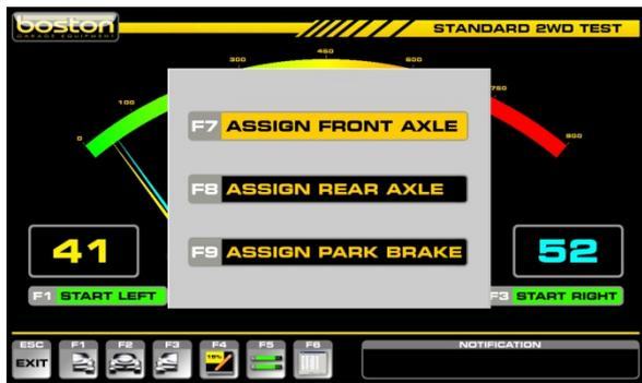
Select F7 to assign all the results from the FRONT AXLE test to memory.
