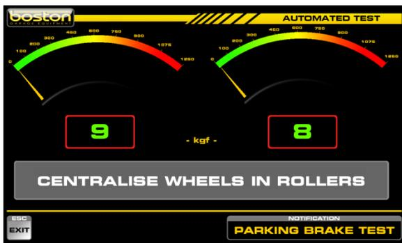
Once the SERVICE BRAKE test is complete the PARKING BRAKE must be tested. With the rear axle still positioned in the roller bed the rollers will re-start.
