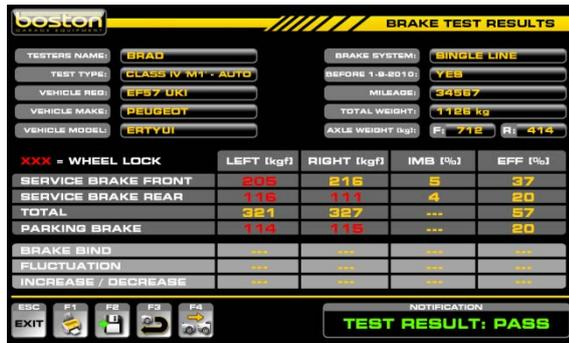
When the user reaches the results page, the software will automatically generate a PASS or FAIL result and the operator can print the results by selecting F1. The software will also save the vehicle details and test data automatically in the internal database. The user has the option to also add the customer's details to the test information by selecting F2 SAVE DATA.
