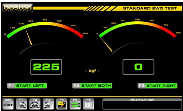
Left roller stopped by the user using the remote control or keyboard. The wheel-lock indicator is not shown but the highest brake force reading achieved is shown in the results box.
