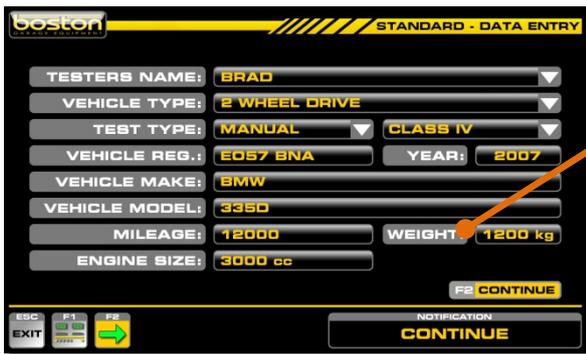
The total vehicle weight should be entered here if the **weighing system is not** fitted to the roller bed.
