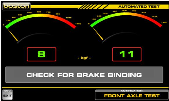
The operator should now check for binding from either wheel.
