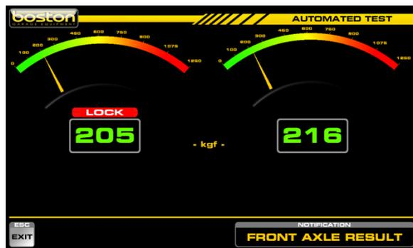
An audible 'bleep' will sound and the operator must now apply the SERVICE BRAKE to max.
