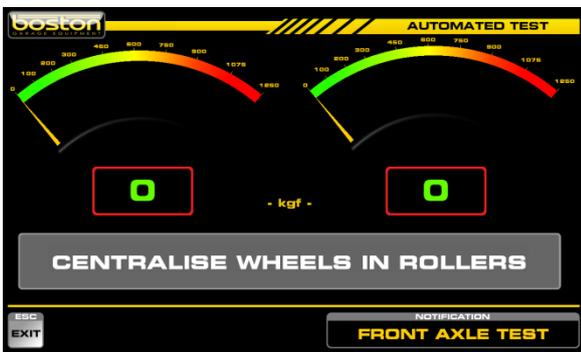
The rollers start and the operator should ensure the wheels are central in the rollers.
