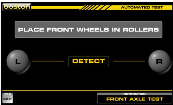
The software will only continue when the wheels are detected in both rollers.
