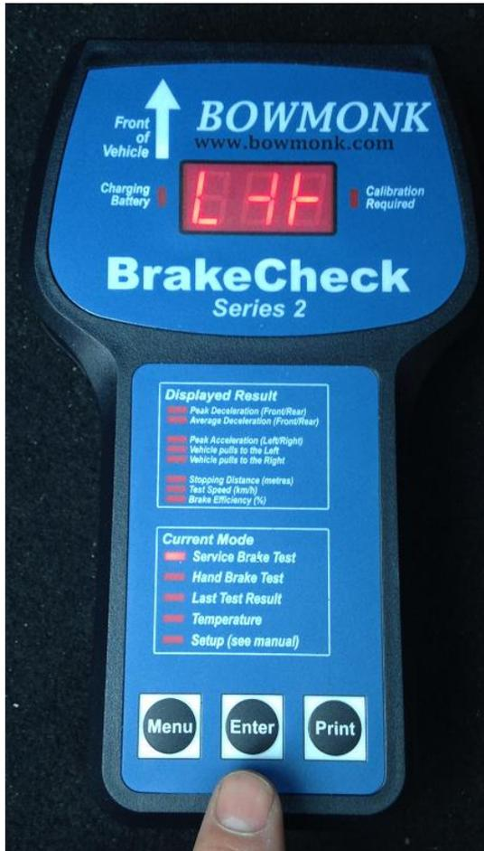
When the unit is positioned level enough to start the test the following symbol will be shown on the display:
