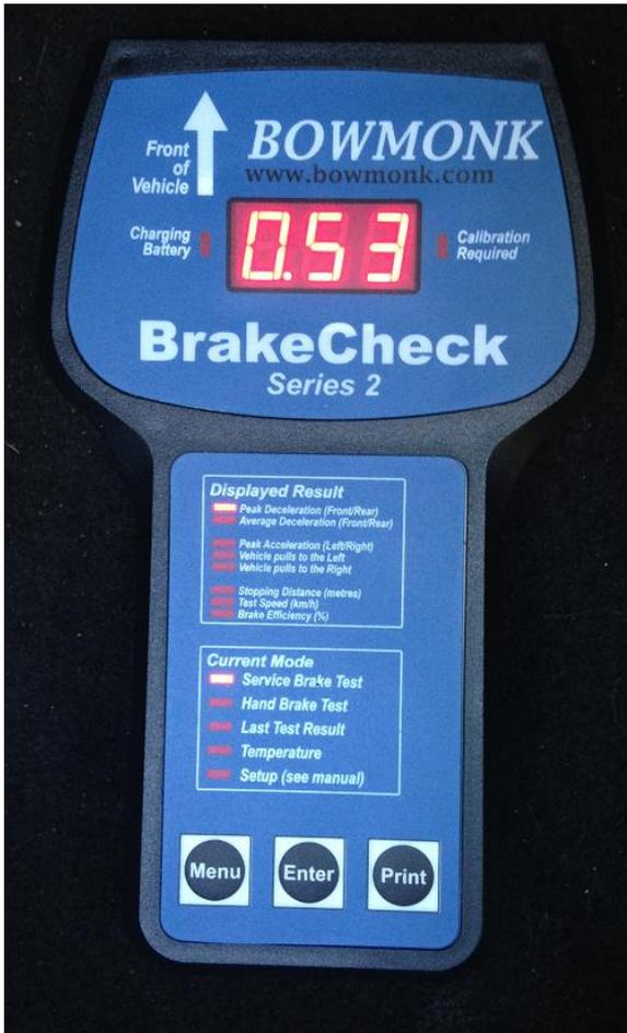
Once the vehicle has been brought to a complete stop, the unit will generate and display a braking efficiency value.
