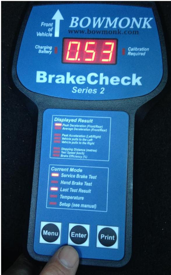
To view the Service Brake test report, press the **Menu** button until the *Last Test Result* and *Service Brake Test* LEDs are illuminated.
