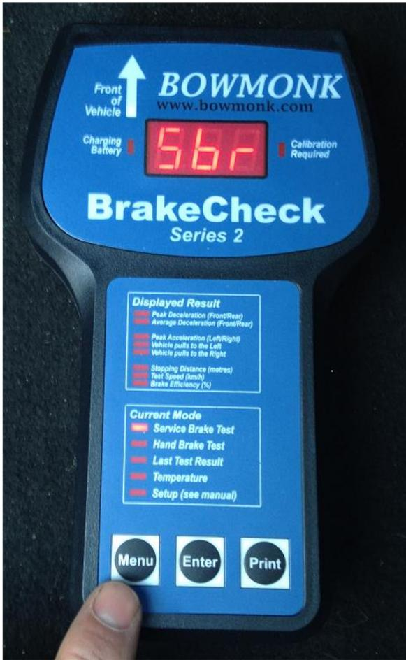
Position the BrakeCheck unit on a level surface, such as the passenger side foot well.
