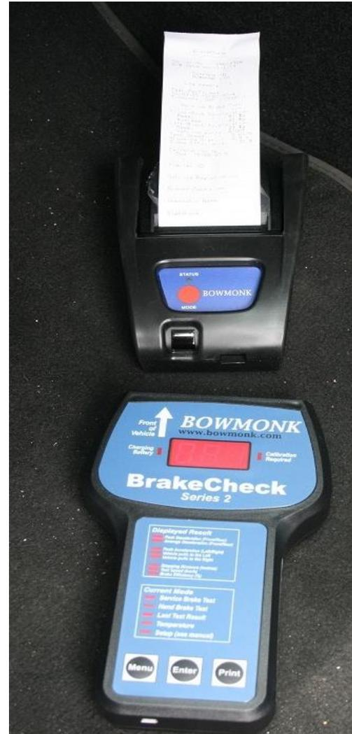
To view or print the Hand Brake test, carry out the same procedure, but use the **Menu** button to illuminate the *Hand Brake Test* and *Last Test Result* LEDs.
