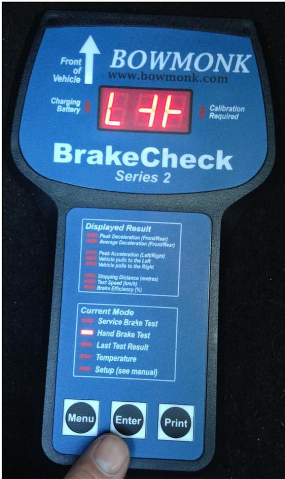
Once the Service Brake test is complete, change to Hand Brake mode by pressing the **Menu** button (so that the *Hand Brake Test* LED is illuminated).
