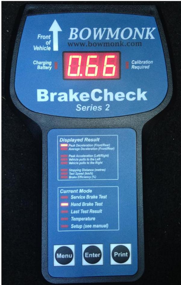
Once the vehicle has come to a complete stop the display will show the braking efficiency of the Hand Brake.
