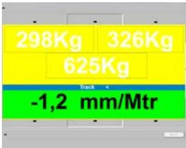
Track measurement for front axle:
