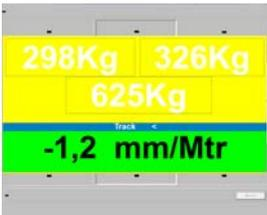
Track measurement for rear axle:
