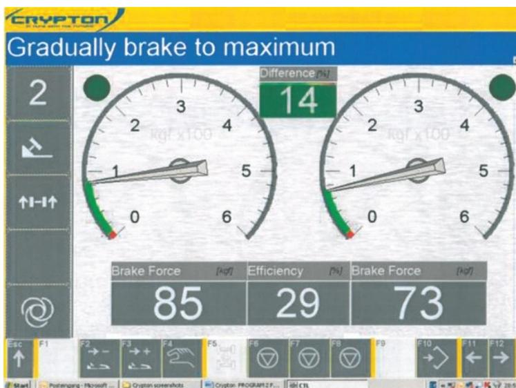
After braking to maximum, either the slip lock out will happen indicated by green lights or once you have achieved maximum braking without any slip lock out, release completely and the maximum results without slip lock out will be shown.
