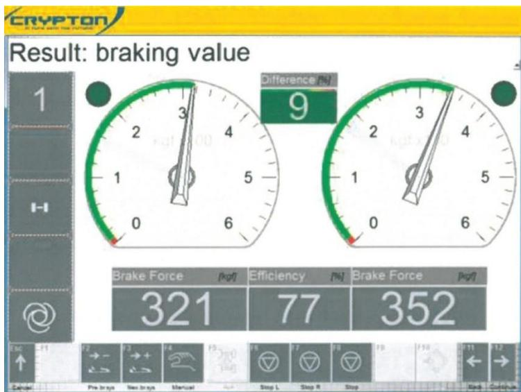
You may or may not slip lock out. If you do, the indicating green lights will come on otherwise you may brake to maximum and then release down to the rolling resistance to allow the rollers to stop, indicating the maximum reading but without slip lock out.
