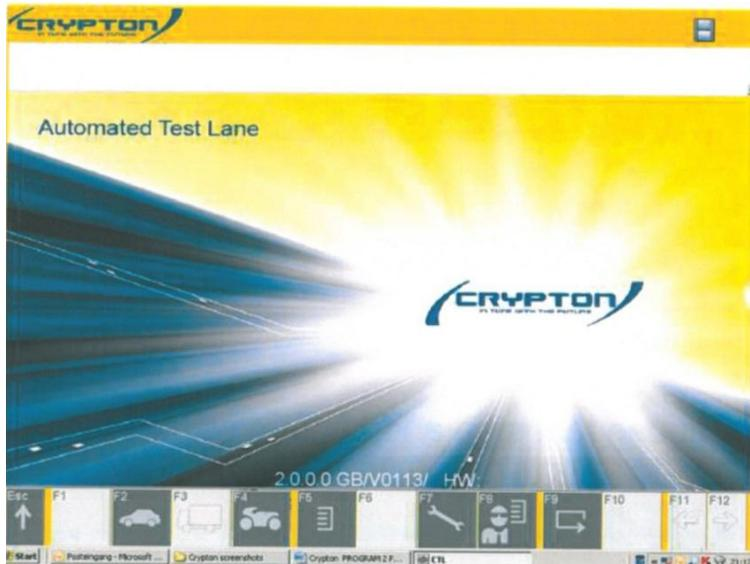
Select F4 to switch to motorcycle testing mode. Note the hand symbol in the left hand information bar to confirm.
