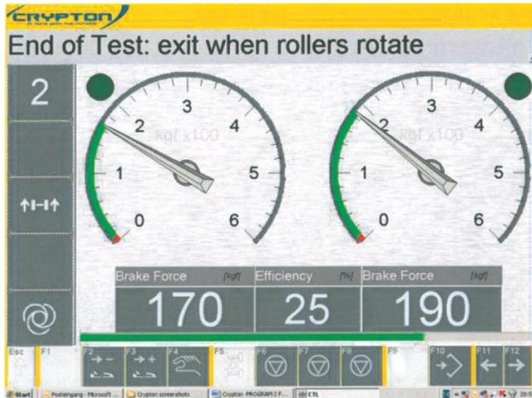
Once all measurements have been completed, drive the vehicle out of the rollers, apply the handbrake and go to the control unit.
