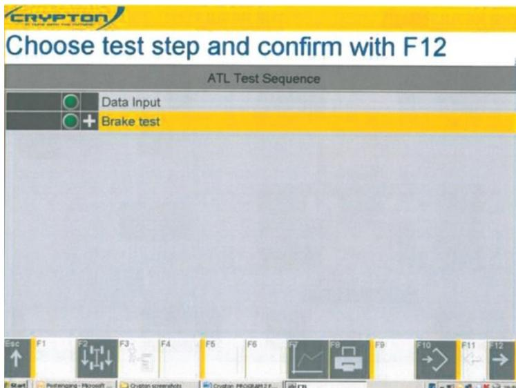
A plus sign next to the brake test means the vehicle has passed according to the criteria. A minus means a fail. There are many ways to view and examine the results as well as to print out various protocols.
