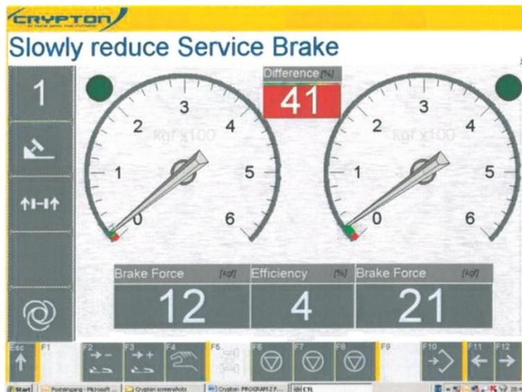
You may reduce the service brake force to the rolling resistance red shaded area, checking for the rate of decrease.
