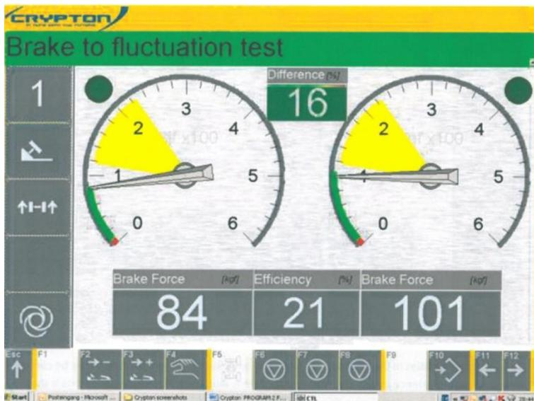
After the rolling resistance has been completed a shaded area is shown in which you are asked to brake to fluctuation test, at which time you should be checking the rate of increase. If you stay within the shaded area, you should not lock out the rollers. If you accidentally do lock out, then this procedure will start again
