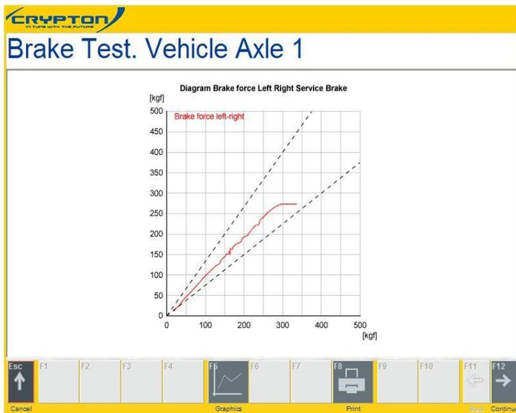
This graph displays the difference in braking force between the left and right-hand wheels. As far as possible, the curves should be regular and situated centrally. They indicate whether a vehicle pulls strongly towards the left or right (front axle) or tends to skid (rear axle) during braking. The dotted lines represent the preset maximum braking force difference. click F12 to view next axle, or F11 to return to previous.
