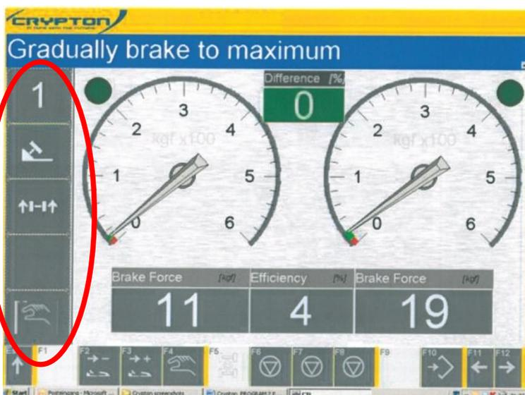
Test printouts will indicate the brake tester locked by placing an asterisk \* in front of the relevant test value.
