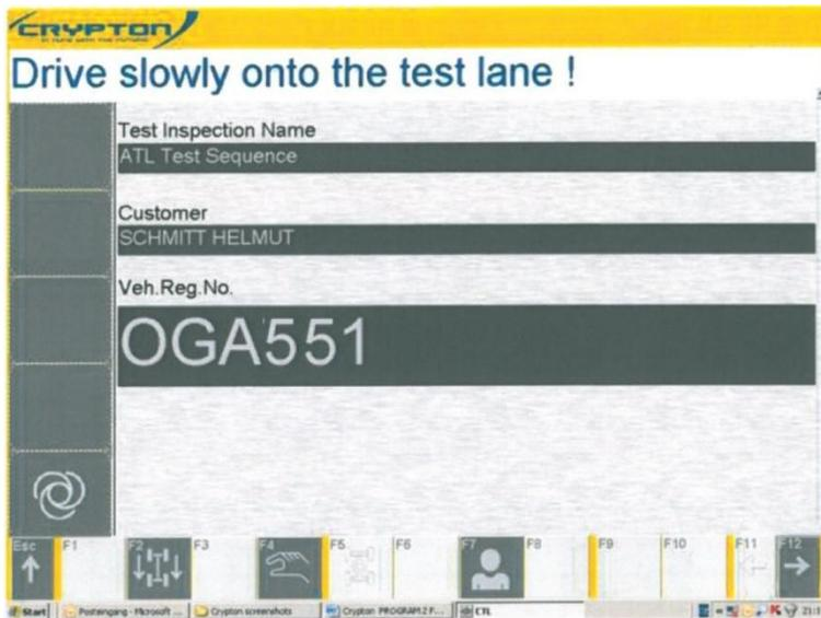
Input data and vehicle details as shown in the automatic procedure above, then select manual mode using the F4 button on the IR remote control. The screen above will be shown with the manual indication (hand) being shown in the bottom left information box. The vehicle can now be driven into the rollers:
