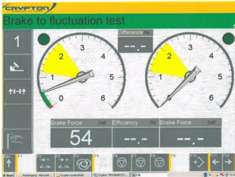
Brake to fluctuation either on left side or both rollers together. You are checking the rate of increase and then holding the needle within the yellow shaded area. After fluctuation test has been carried out, release the brake (s) so the needle drops to the bottom, checking the rate of decrease.
