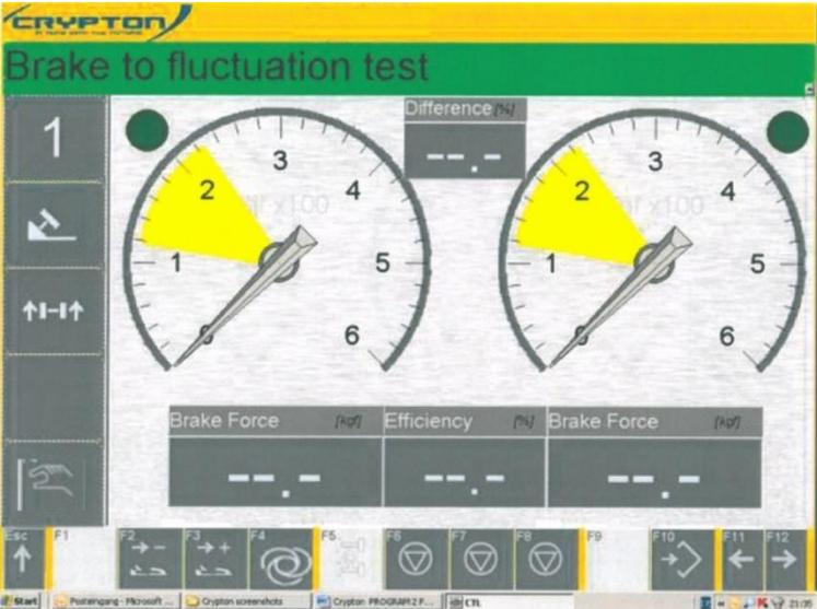
Once the rolling resistance is shown and the vehicle is squared, press F8 on the IR remote control to stop both rollers.
