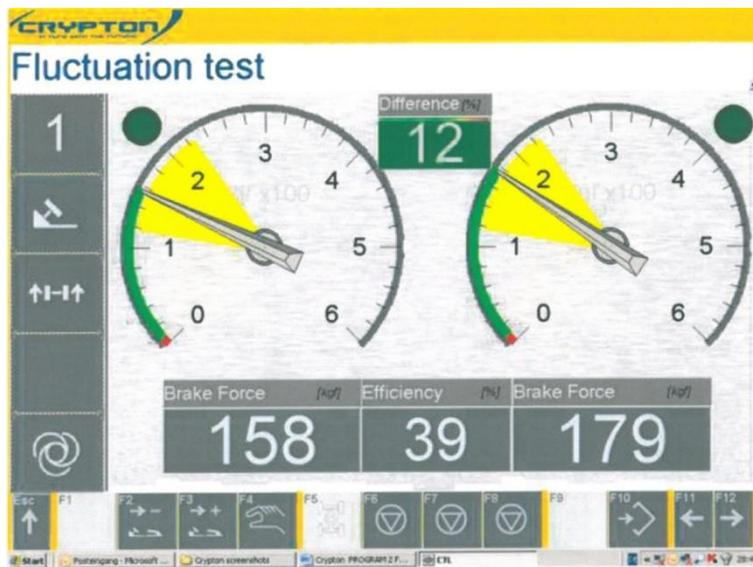
By holding the needles in the shaded area as steady as possible, a fluctuation test may be carried out. The maximum difference during the whole procedure is indicated. The deceleration box is the percentage of deceleration shown during braking.
