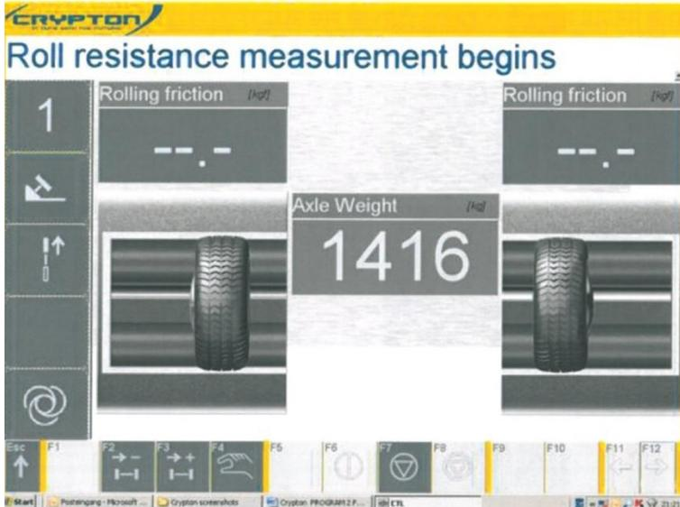
Using the remote control, start the roller by pressing F6 (left) or F7 (right) as required.
