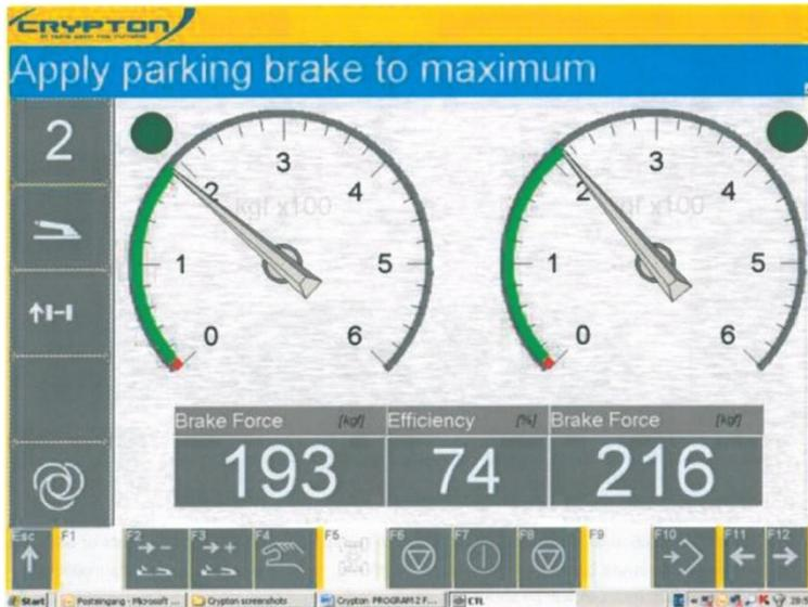
With both rollers rotating at the same time, follow the instructions and brake gradually to maximum. Due to the severity of some parking brakes, the vehicle could roll backwards out of the rollers before full braking has been achieved. If this happens the rollers will stop rotating. Let the vehicle roll back into the rollers by letting off the parking brake.
