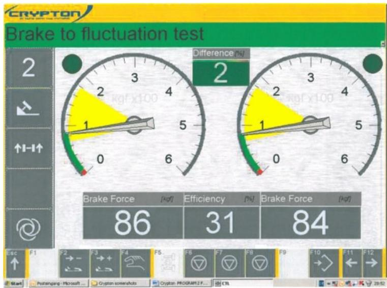
Apply service brake to fluctuation checking the rate of increase. Note that there is also an imbalance displayed on the second axle which is recorded at maximum braking for the MOT rear axle test results.
