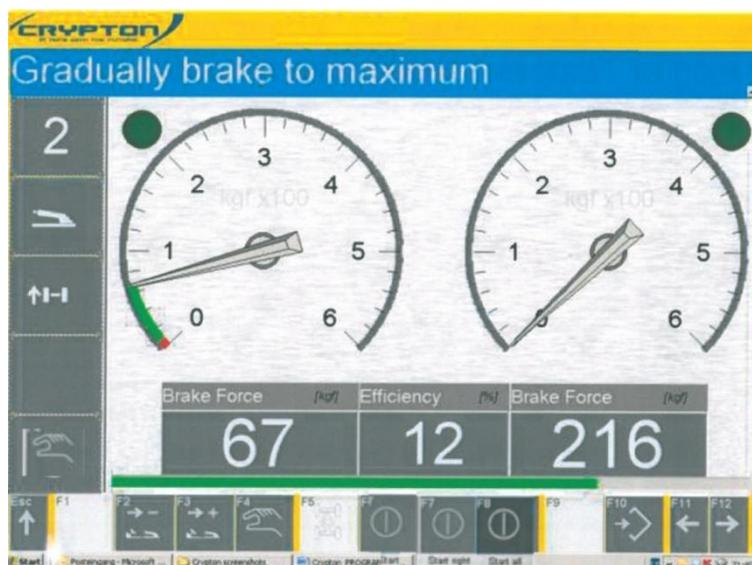
Press F3 to move from service brake to parking brake.
