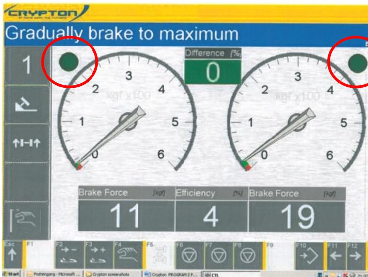
Where slip limits are achieved the brake tester will automatically 'lock'. Visual indication is provided by the green indicators above the dials. When slip is achieved and the brake tester 'locks' the indicators colour will change to light Green.
