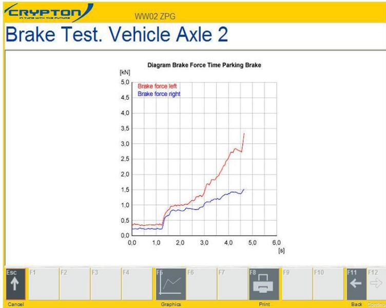
The graphics will show the parking brake over a period of braking time. The red line is the left side, and blue the right.
