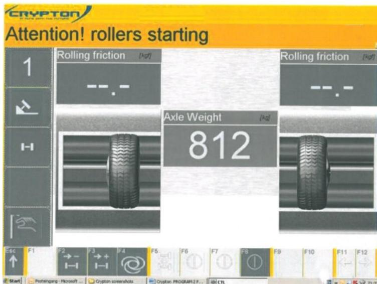
Once the vehicle is in the rollers Press F8 to start both rollers together in order to straighten up the vehicle and start the rolling resistance readings. The left roller will always start up first in sequence.
