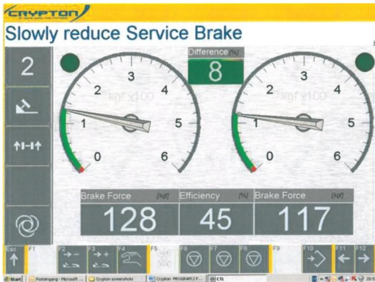
Reducing the brake force and checking the rate of decrease.
