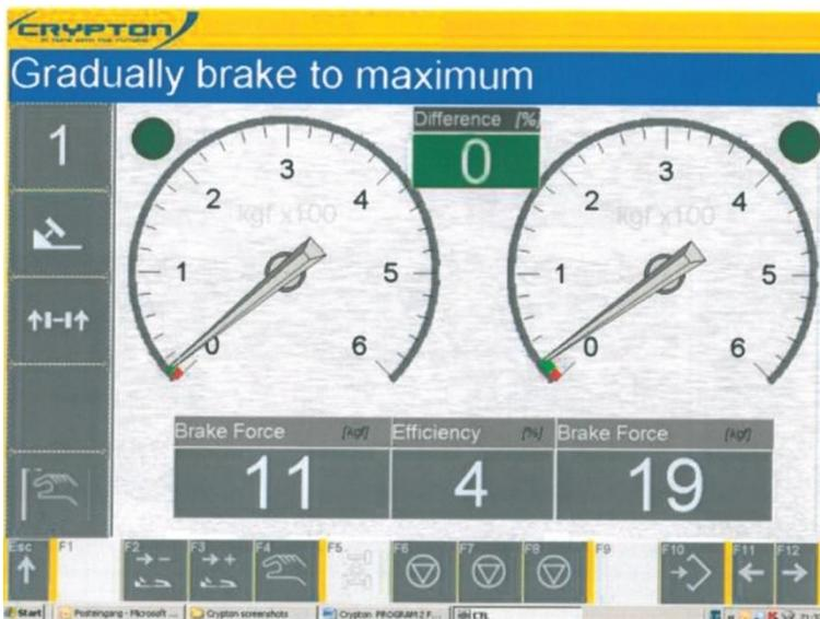
Pressing F6 left side, F7 right side or F8 both sides, brake to maximum. You will either lock out with the green light illuminated or no lock out occurs in which case you can release the brakes and the roller (s) will stop giving the maximum reading. Otherwise you can press F10 at the maximum reading when the result will be recorded and the rollers will stop.
