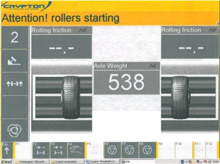
Rear axle is in the rollers, axle weight is shown and they are about to start up
