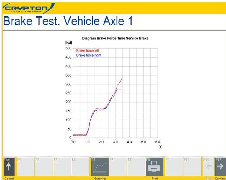
The graph shows braking force over time. The left-hand side in red and the right-hand side in blue. You can click F12 to view next axle, or F11 to return to previous.
