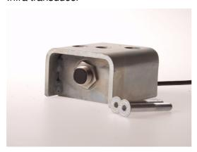
Due to light-reflecting sticker fixed to the tyre the infra cyclometer is able to sense the turns (it counts ten rotations). The given values are trasmitted to the central unit as well. In case of analog tachograph device, the cables belong to the tachograph's type have to be used to the test.
