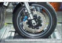
Car brake testers can be easily retrofitted for motorcycle tests.
