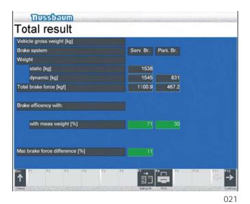
You can return to the screen for test procedure overview by pressing the F1 ESC key.
