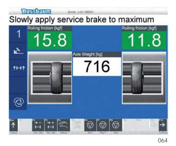
After the slip limit cut of has been achieved or 5 seconds has elapsed, decrease the force on the brake pedal.
