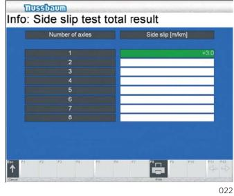
The side slip measurement results are shown in m/km of the front (axle 1)and rear (axle 2) axles. This value indicates the axle offset to the left or right of a vehicle in metres, which it exhibited following a drive of one kilometre with no correction to the steering.
