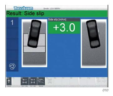
The front alignment plate eliminates disturbing lateral forces (strain) in the tyres. The next plate measures the wheel misalignment.
