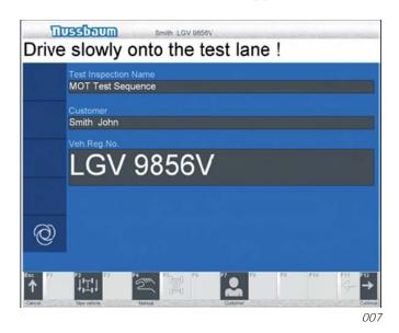
The "Test line main screen" re-appears on screen. The information you have entered is now displayed in the "Customer" and "Reg. number" fields. You can now commence the test.
