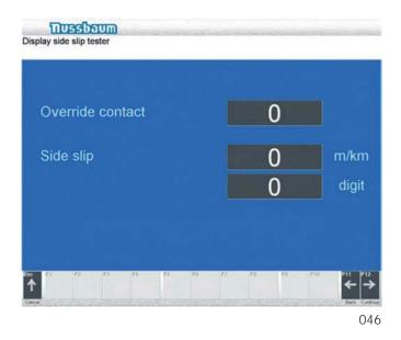
Under unloaded conditions the value should be around 0.
