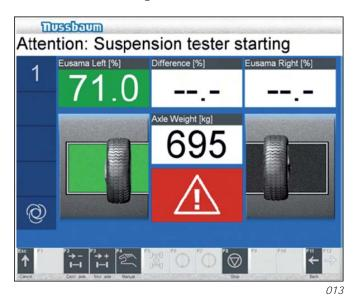
The platform begins to oscillate in order to determine the road adherence versus the frequency. To this aim, the motor is revved to its maximum frequency, switched off and measured while it is coasting.
