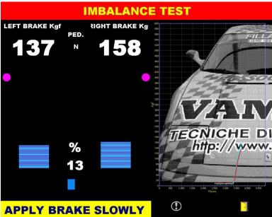
According to the VOSA MOT Test procedure, a braking force up to 75% of the maximum is applied before test ends.
