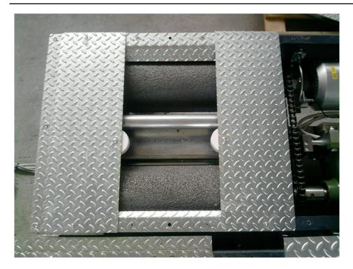
Remove the central plate of the class I, II and III adapter.
