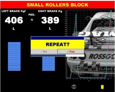
After that the same testing sequence applies to the rear axle: maximum force, bind, imbalance.
