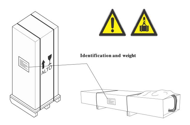
Handling must be carried out through transpallets or fork-lifts. The fork lifting points are the cavities provided on the pallet. There is no need of lifting the machine in special positions. The Roller Brake Tester is in turn coated with protection cardboard, wrapped in plastic strap and put in wooden crates. Sizes of packing 2570x830x550, approx. weight 400 Kg.
