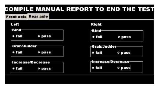
The operator is now requested to select/adjust pass/fail result on each and every single. Such a results window show at the end of every axle test; the operator is responsible to select the result according to his/her judgment of the condition of the braking system of the vehicle tested.
