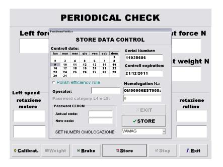
Verify that the date is correct (1) and enter the serial number of the bench (3), type the expiration date of the next inspection (4), generally one year after installation. Enter the name of the engineer (2) that carried out the verification.
