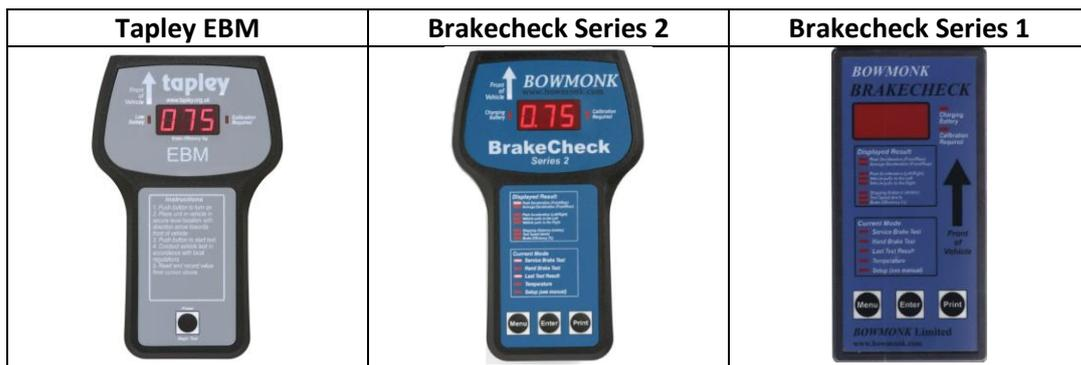
User Manuals for the Tapley EBM and Brakecheck decelerometers shown above are provided on the USB 'Thumb Drive' supplied with your Bowmonk Connected device.
