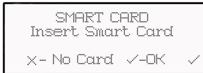
On the 'Insert Smart Card' screen, press the tick key to confirm. Data will then be read from the smart card to the OmiSmoke.
