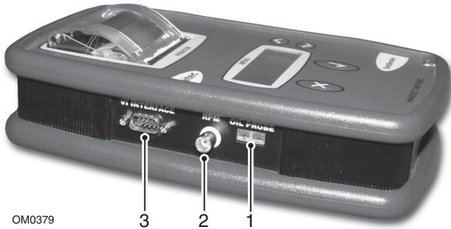
1. Engine oil temperature sensor connector
