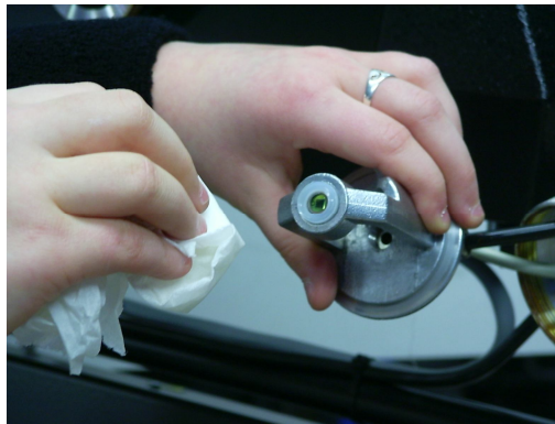
Figure 7. Cleaning the receiver of the smoke meter.
