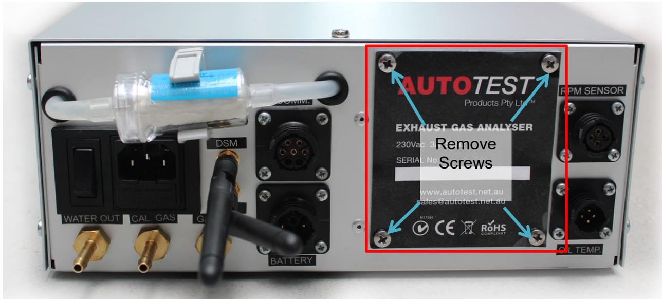
Figure 38 Remove Screws from Case
