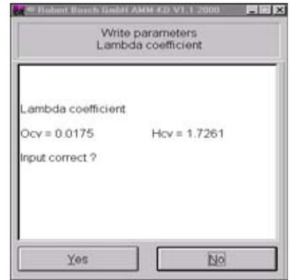
The **OK** box is displayed for approx. 1 s. The  $HC_v$  and  $OC_v$  values are stored in the exhaust-gas analyzer.
