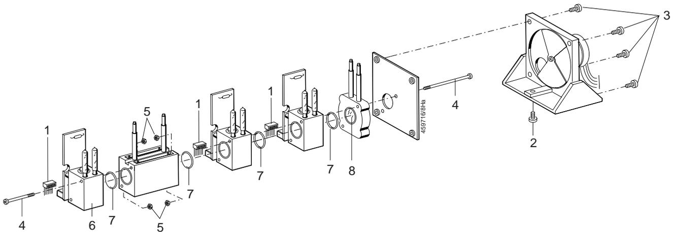
! On assembly, take care to ensure that the sealing O-rings (7) of the analysis chambers are properly seated in the groove and that the windows (8) of the analysis chambers are in the recesses provided.
