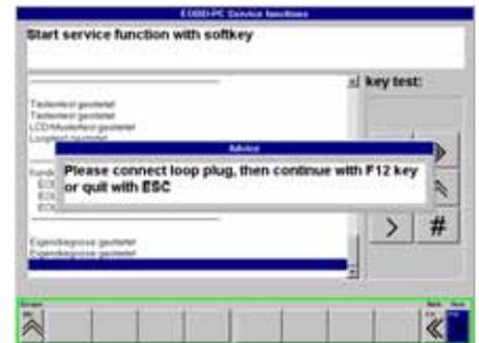
If the loop test has been concluded with no errors detected, the message: BsTest "Loop" "TFau" \$0000 "TSchr". appears. Of importance here is the digit after "TFau" (TFau = Type of **F**ault). If the self-diagnosis revealed no faults, this must appear as \$0000. For error messages see Section 4.4.5.3, Error messages.
