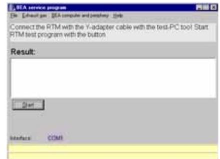
When the Service program starts, you can view the software version, checksum, RTM mode and dip-switch settings via the different menu items.
