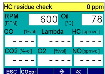
6.2 Checking oil temperature and engine speed in Petrol Diagnosis
