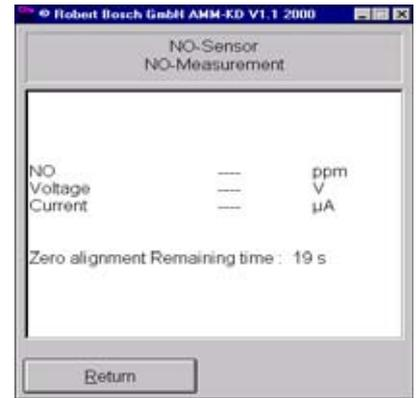
After zero calibration, the data of the NO measuring sensor are displayed.
