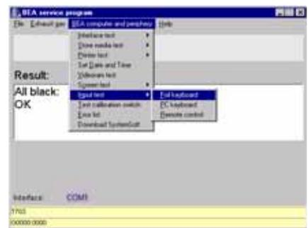
Press membrane keys ESC, F1, F2, F3, F4 and F5 one after the other.
