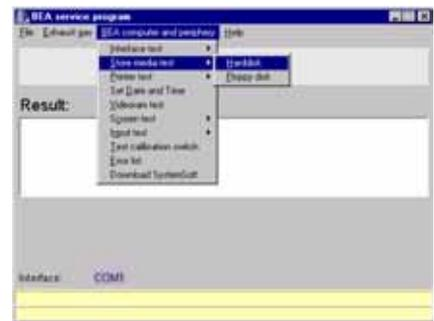
The hard disk test is executed automatically.
