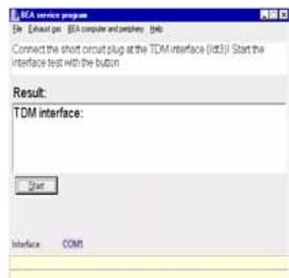
If the interface test is error-free, the message **OK** appears in the results box. If the interface test is unsuccessful, an error message is displayed.
