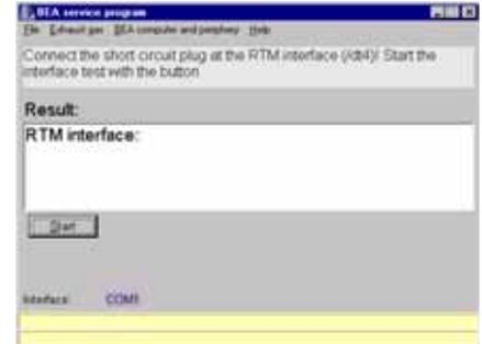
If the interface test is error-free, the message **OK** appears in the results box. If the interface test is unsuccessful, an error message is displayed.
