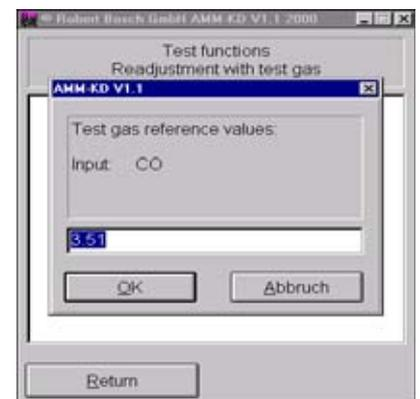
Using the keyboard, enter the calibrating-gas values for **CO<sub>2</sub>** as stated on the certificate.
