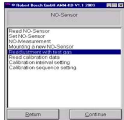
Using the keyboard, enter the calibrating-gas value in **ppm NO**.
