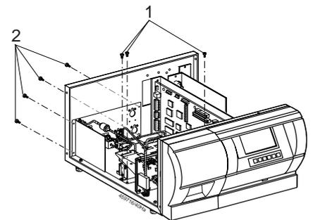
3. Pull the exhaust-gas analyzer module approx. halfway out of the BEA.
