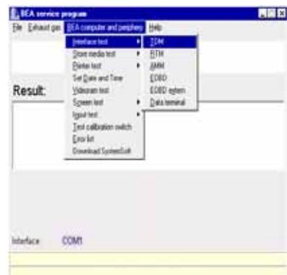
Remove the 20-way Micro-Match plug from X8 of the control module PCB. Plug the 20-way shorting plug into X8 of the control module PCB. Start the interface test by double-clicking the mouse or pressing Enter ↵.
