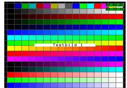
If the geometry image is in order, then the Service software image displays the following reference:
