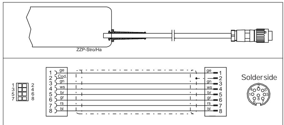
6.5.2 Terminal diagram of TD/TN connection cable
