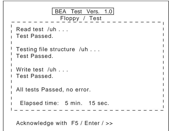
In the event of a fault the floppy disk has to be replaced (see chapter 10.22).
