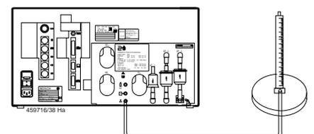
6. Connect the flow meter (rotameter) to the measurement gas intake of the BEA (see diagram).
