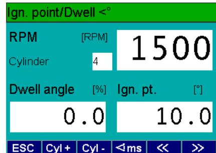
9. Repeat the test with an ignition point of 60°crankshaft
