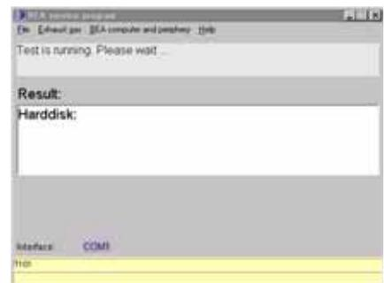
If the hard disk test is error-free, the message **OK** appears in the results box.
