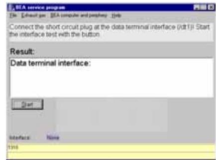
If the interface test is error-free, the message **OK** appears in the results box.
