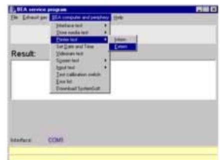
5.11 Checking the external printer
