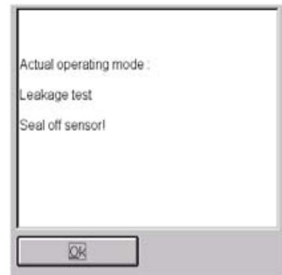
The pump is then switched on and off in cycles over a period of approx. 3 sec. until a certain level of vacuum is reached. After this, the exhaust-gas analyzer module measures the drop in pressure over a period of 15 s. The time is counted backwards from 15 s to 0.
