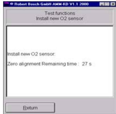
10. Following correct O<sub>2</sub> calibration the new data are displayed.
