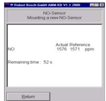
After calibrating gas has flown through the BEA, the measured NO value, the corresponding test current and the date of calibration are displayed.
