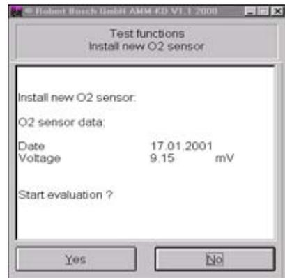
If there is a fault during calibration, this is displayed in plain text. In this case, repeat calibration. The O<sub>2</sub> sensor may need to be replaced again.
