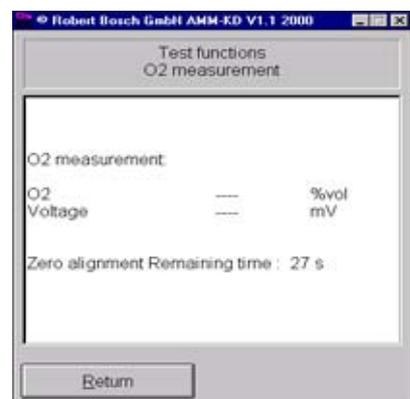
After zero calibration, the pump is switched off.
