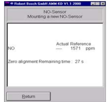
Allow calibrating gas to flow through the BEA in line with the instructions on screen.
