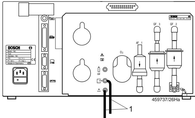
i If the outlet hoses are shortened or lengthened, calibration must be performed again. The signal from the NO measuring sensor is very sensitive to vibrations from the pump. The strength of these vibrations depends upon the length of the outlet hoses. Following successful calibration, the timer for monitoring the set recalibration interval is started.
