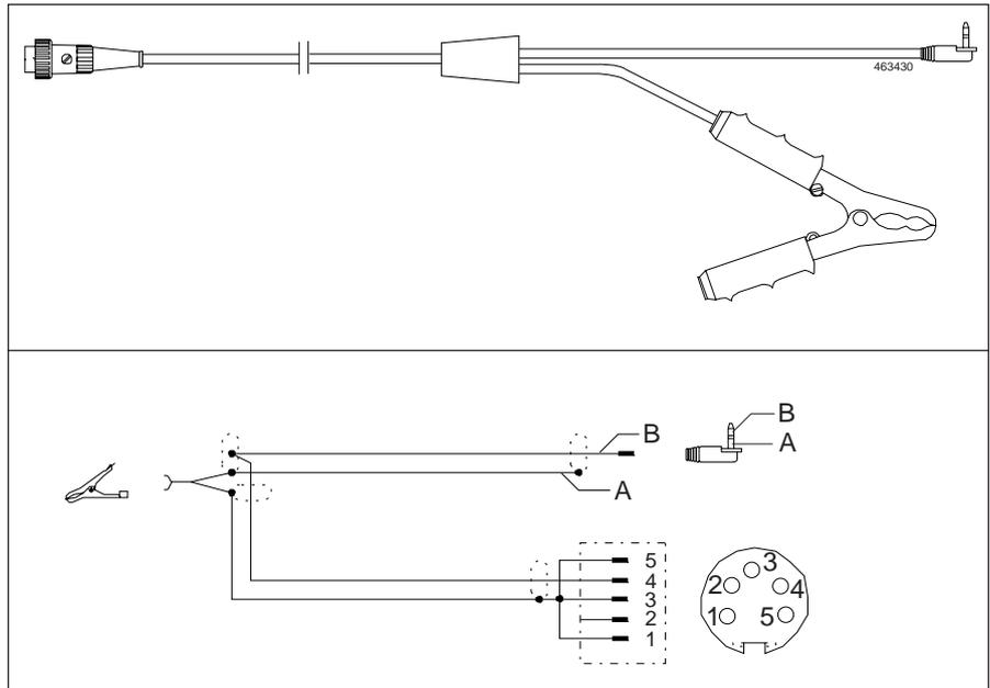
6.1.2 Terminal diagram of temperature sensor
