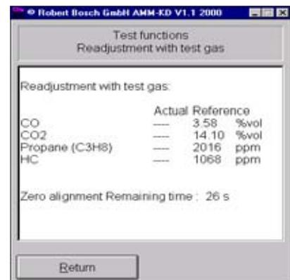
After zero calibration, push the calibrating-gas hose onto the calibrating-gas inlet.
