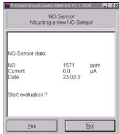
Using the keyboard, enter the calibrating-gas value in **ppm NO**.
