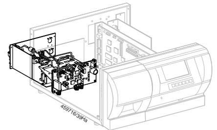
5. Remove the O<sub>2</sub> measuring sensor (3) from the rear of the exhaust-gas analyzer module.
