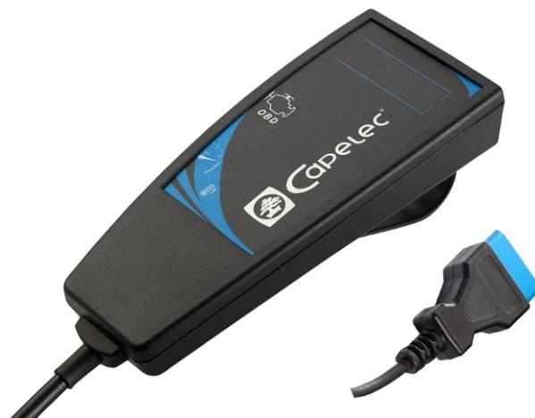
The Scantool is a tool allowing access to the internal data of on-board systems. It connects to the OBDII auto diagnostic plug (SAE J1962 standard) of the vehicle and scans the information stored in memory or current data made available and accessible by one of the 5 standardized protocols.
