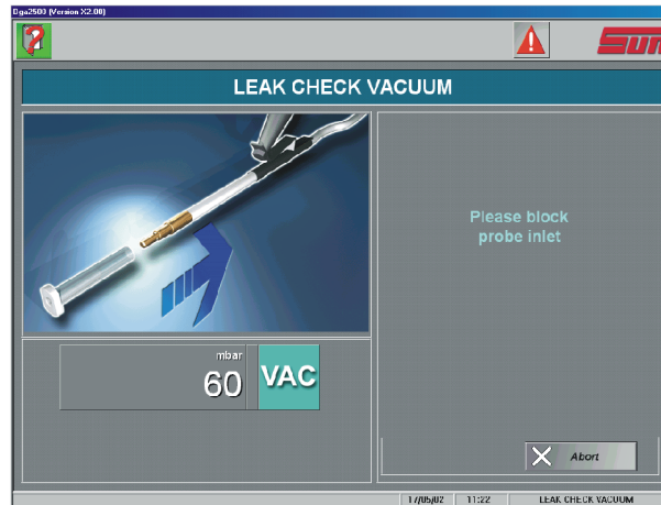
Figure 10-1 Leak Check (Vacuum) Initialization
