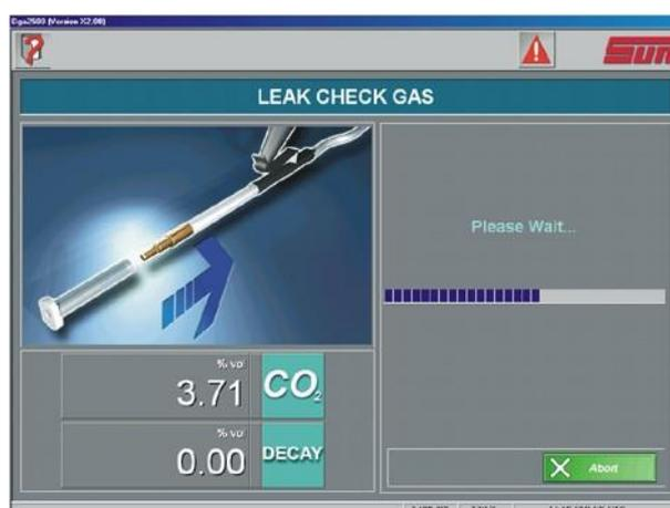
Figure 9-6 Leak Check (Gas) - Measurement
