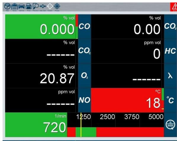
Figure 8-1 The Free Measurement Screen
