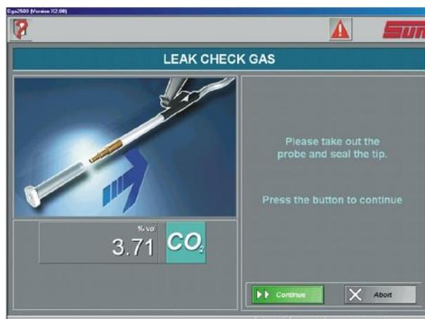
Figure 9-5 Leak Check (Gas) - Block Probe Tip
