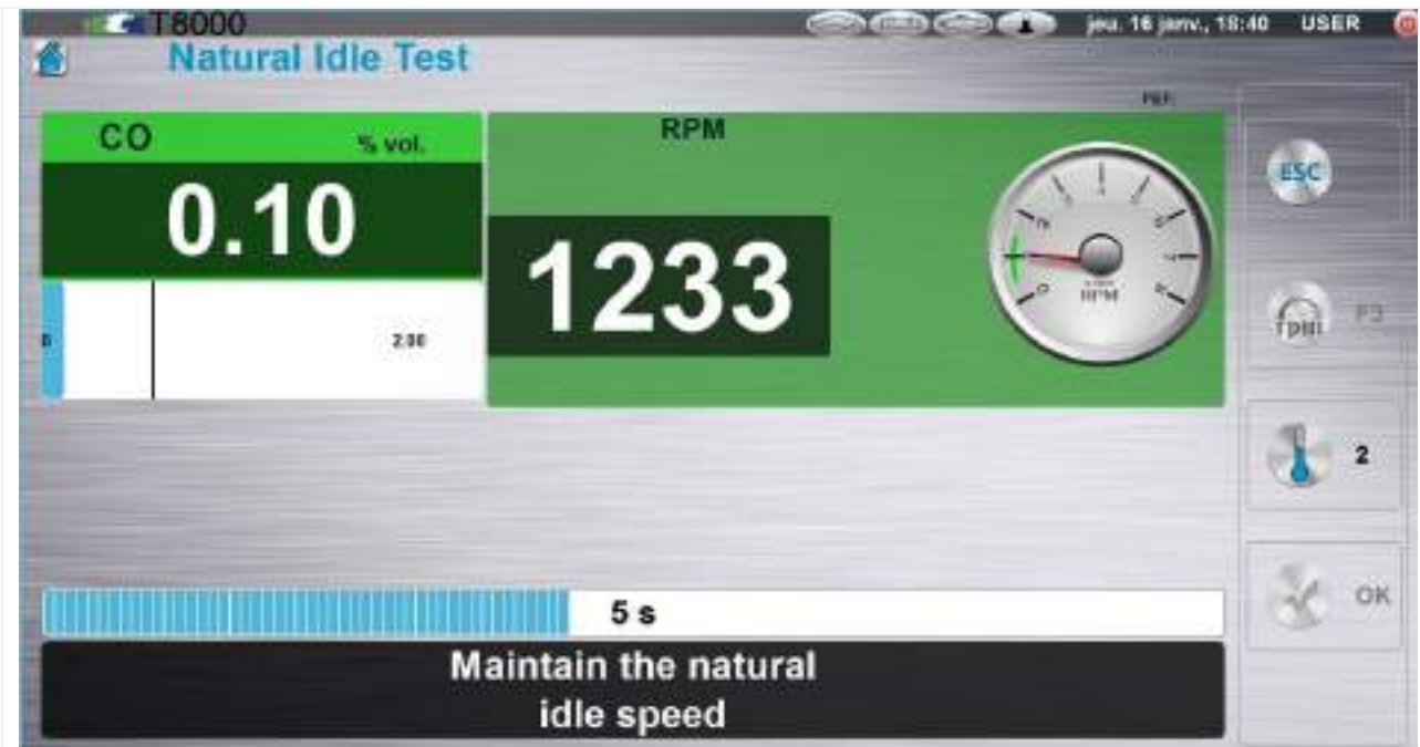
Figure 6.3.8.1-3: Natural Idle speed needs to be maintained during 30 seconds The Natural Idle test will end either when the CO value is within limits or at the end of the 30 seconds countdown.
