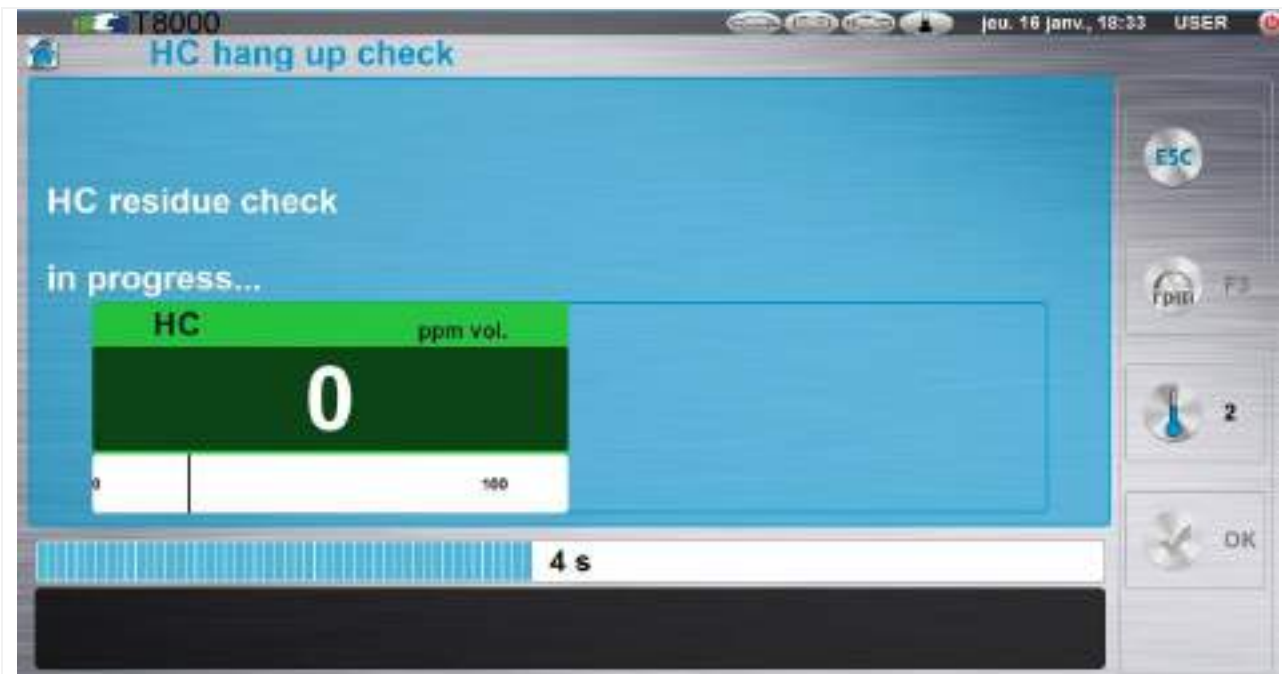
Figure 6.2.4.1-6: Operator is prompted to start HC residue check
