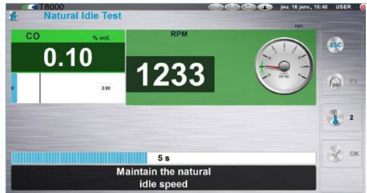
Figure 6.3.8.1-1: During 10 seconds the operator is prompted to adjust the speed to natural idle
