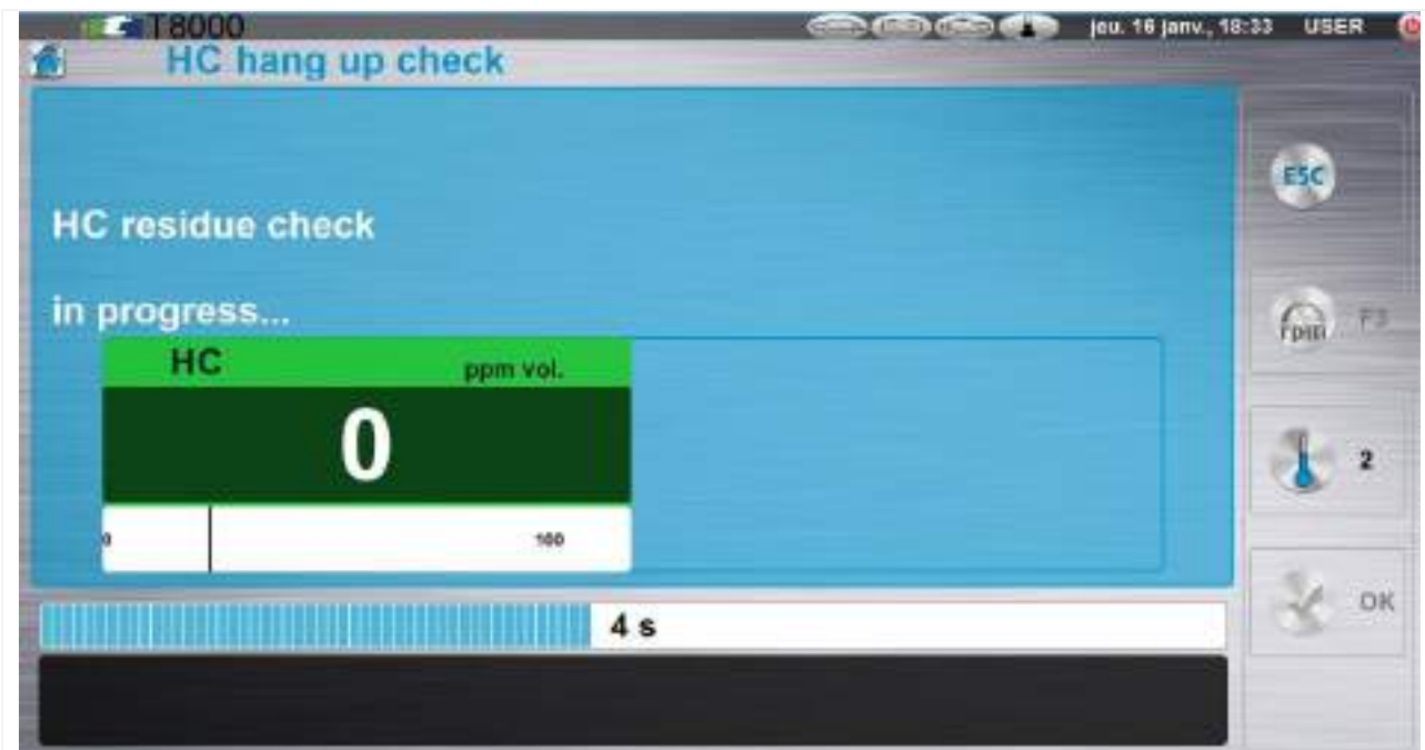
Figure 6.2.4.1-8: HC residue check in progress
