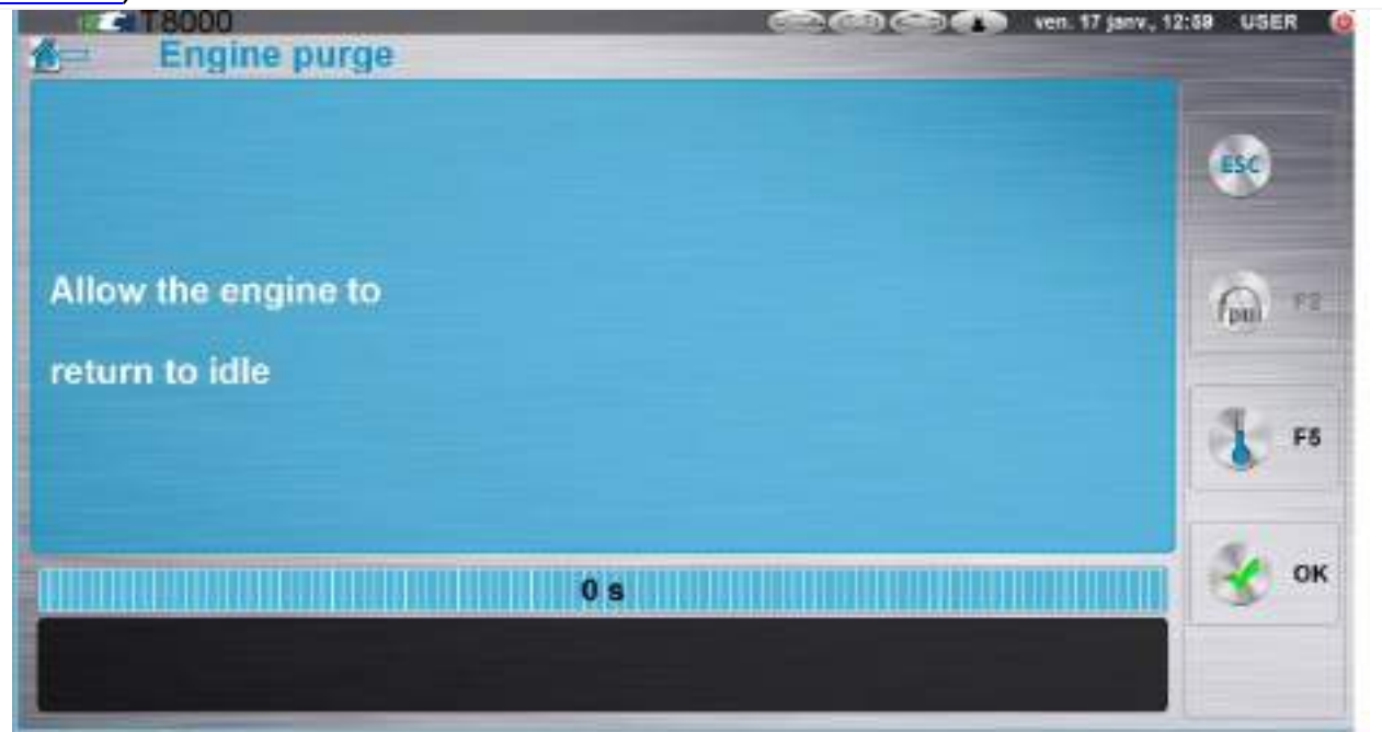
Figure 6.3.8.2-3: The operator is prompted to allow the engine to return to idle
