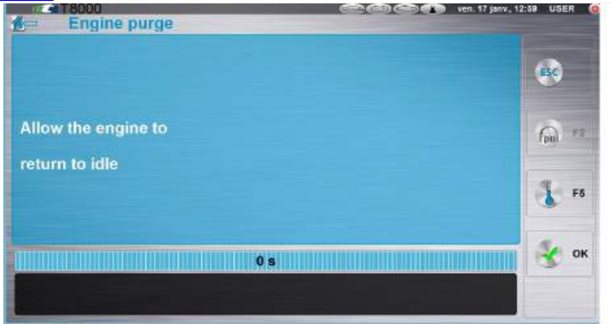
Figure 6.3.8.2-4: The operator is prompted to allow the engine to return to idle
