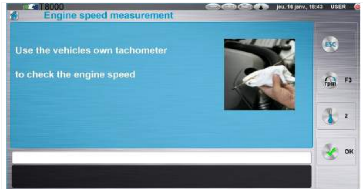
Figure 6.2.4.2-2: On start of Fast Idle test the operator is prompted to use vehicle tachometer to check the engine speed
