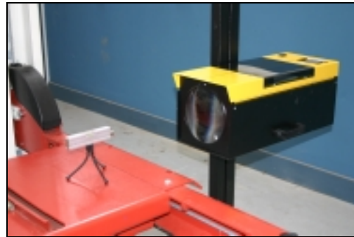
'Place the laser on a level platform'
