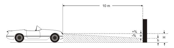
Angle of inclination of light-dark limit against the test surface.
