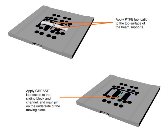
After the monthly maintenance is complete, replace the moving plate and ensure that it is tightly secured. On a regular basis the oil reservoir inside the pedestal should also be checked. The level should always remain the same, but in the event of any leaks this may change. For service and repair always contact your local distributor.
