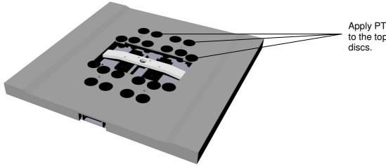
Apply PTFE lubrication to the top surface of all discs.
