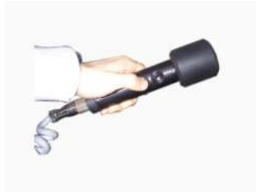
Pic.8 Press the button to start the cycles with the left right play detector.
